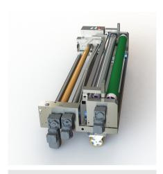
The Ascending Batch Winder can be used for winding and unwinding applications. Especially large and heavy rolls of cloth can be handled in an Ascending Batch Winder because the tubes with cloth are supported in the full width and tension in the cloth is controlled through dancer bars that have an adjustible weight. The required speed of the winder is automatically adjusted through the control system with frequency drive system.
